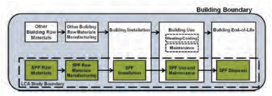
Figure 2-1 Life cycle flow diagram of SPF insulation products
