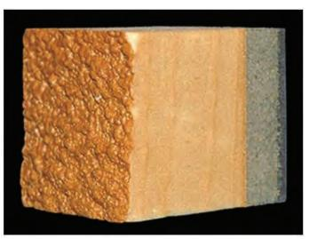
Figure 2-2 Cross-section of spray foam insulation with layers of various densities (collectSPACE.com)
